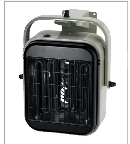
The thermal protector automatically disconnects the unit in the case of overheating. They have a manual RESET button, situated at the top of the housing to reconnect the unit. They also have a switch that allows the thermostat to act on both the fan and the heater element or only on the heater.
